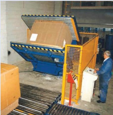
The RR can also be sited 'off-line'. The picture to the left shows how loads of boards which need turning can leave the main conveyor route, enter the RR and then return to it after inversion.
