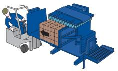
3 The clamping table rises and a second forktruck (fitted with platens and a pull-push) approaches from the side. The driver powers a moving side wall on the inverter which pushes the load onto his platens.
