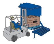
The inverter is loaded with the materials on the pallet you want to retain.
