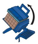
**2** At the push of a single button the pallet is gripped hydraulically, the load clamped and the inverter revolves through 180°.
